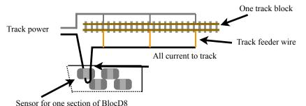
Locomotives, lighted cars and rolling stock with resistive wheels sets draw different amounts of current from the track. The BlocD8 has two potentiometers to adjust sensitivity. Turning the pot CCW will increase the sensitivity. **If the pot is turned fully CCW there may be false block detection**. Passing the feed wire through each sensor two times will increase the sensitivity and can improve reliable detection. See "TIP" in section 2.
