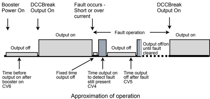
If there are several DCCBreaks on the layout, they can be programmed so that each has a different turn on time after the booster turns on. This prevents the booster from experiencing the total layout load current at power on.
