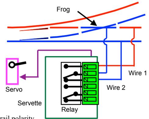
The relay wiring shown is very close to the actual except for Wire 1 and Wire 2. These wires may have to be reversed at the relay terminals so that the correct rail polarity gets to the frog. This will be determined by the way the servo is mounted and linked to the turnout. Either set of relay contacts can be used for frog power.
